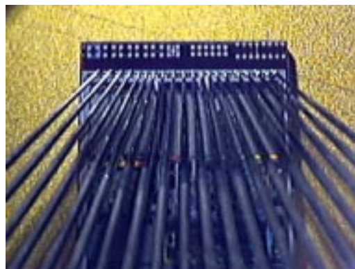
Fig. 8.4: Probecard lowered onto the SMC
