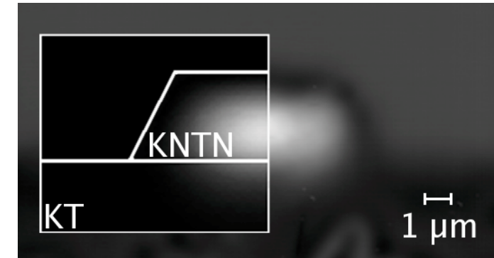
Figure 4.5: Waveguide profile and TE mode intensity distribution of \lambda = 1579 nm laser light propagating in a potassium sodium niobate tantalate thin film ridge waveguide. Left inset shows simulated mode profile with excellent agreement to measurement.
